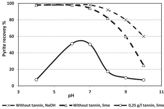
Fig. 2. Effect of pH on depressing action of tannin, along with curves recovery-pH using different modifiers (CaO, NaOH).
