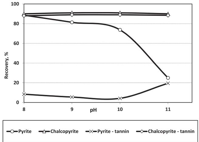
Fig. 4. Comparison between pyrite and chalcopyrite, with and without tannin.
