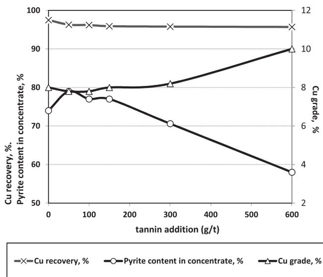
Fig. 6. Effect of tannin addition on a disseminated copper ore flotation.
