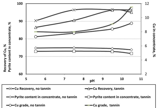
Fig. 5. Effect of tannin on disseminate copper ore; tests at different pH, with and without tannin.
