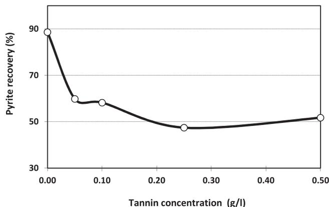
Fig. 1. Effect of tannin concentration on pure pyrite flotation.
